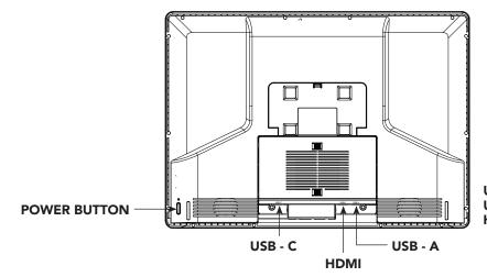
**USB - A** (Device Charging / Software Update) **USB - C** (Ethernet in) **HDMI** (HDMI in)
