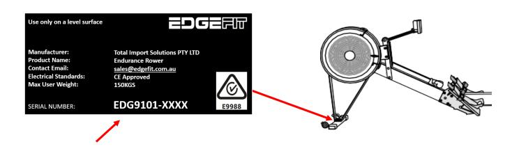
Serial Number is located here on the front foot stabilizer.
