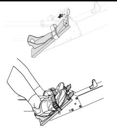
To set the Flexfoot, pull the toe piece toward you to release the Flexfoot from the two pegs. Slide the toe piece up or down to achieve the proper setting, then press the toe piece back down onto the pegs.
